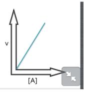
$\mathbf{A}$  is the x axis . The V is y axis & the slope of the line is the  $\mathbf{K}$
