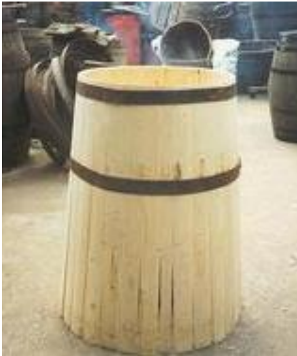
Barrel under construction
